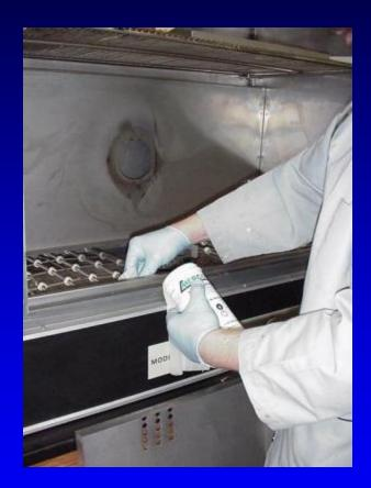
Sulfur impregnated cloths may be used for a final wipe down of the area being cleaned
