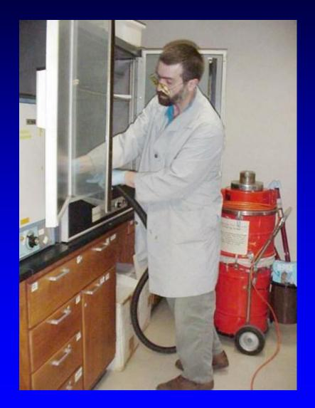
One can use a special vacuum cleaner is available which is designed to pick up mercury droplets safely.
