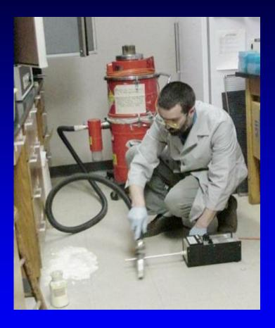
Air monitoring should be used in conjunction with the mercury vacuum to ensure the complete removal of mercury and to assess spill cleanup personnel exposure.
